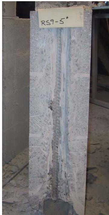
**Figure 6.** Wall cross-section with Oztec Rebar Shaker consolidation
