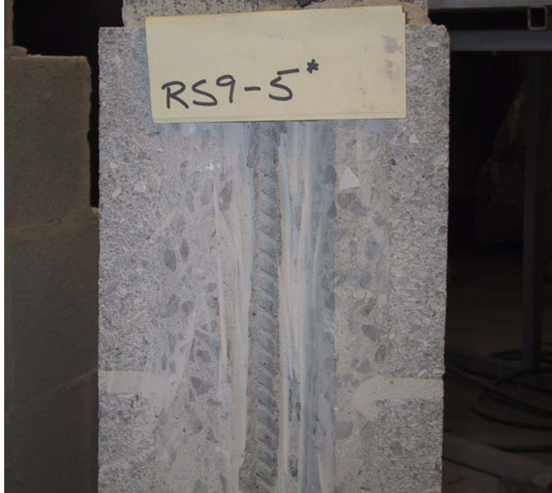
Figure 7. Wall cross-section with Oztec/Rhodes Rebar Shaker consolidation
