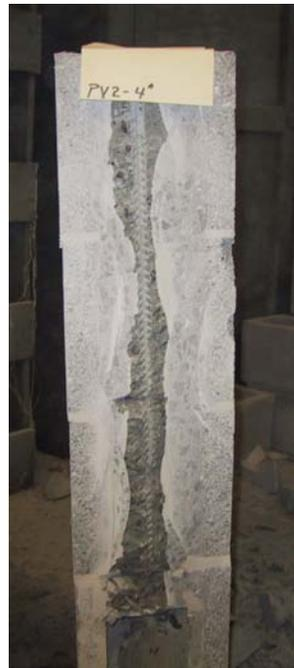
**Figure 4.** Wall cross-section with pencil vibrator consolidation
