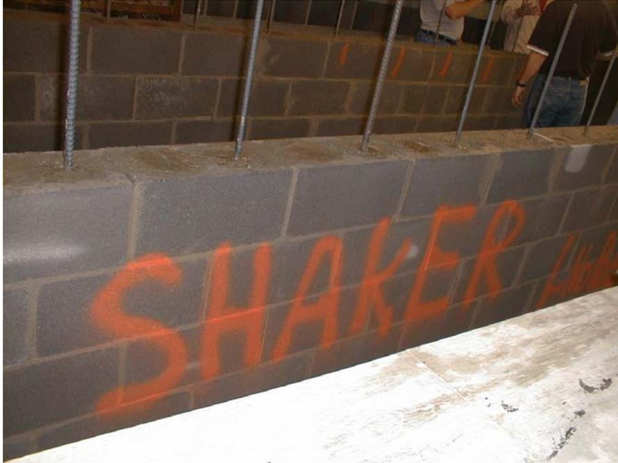
**Figure 1.** Completed wall prior to testing
