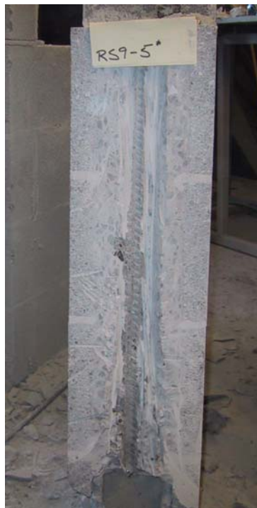
Figure 6. Wall cross-section with Oztec/Rhodes Rebar Shaker consolidation
