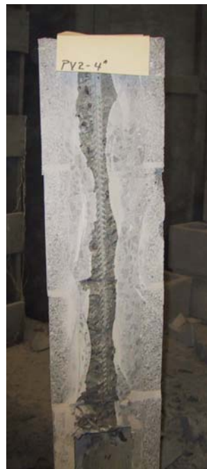
Figure 4. Wall cross-section with pencil vibrator consolidation
